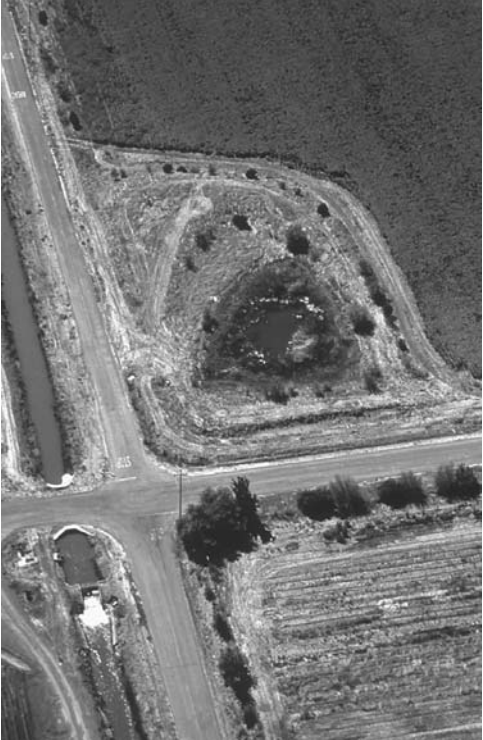
Figures 8.13a–b A, right: Farmer John Anderson's two-stage tailwater pond traps sediment in the first, oblong pond, then returns the water to the second, habitat pond, shown at eye level in B, below . Tailwater ponds achieve multiple conservation functions for valley agricultural fields. Photographs by John Anderson.
