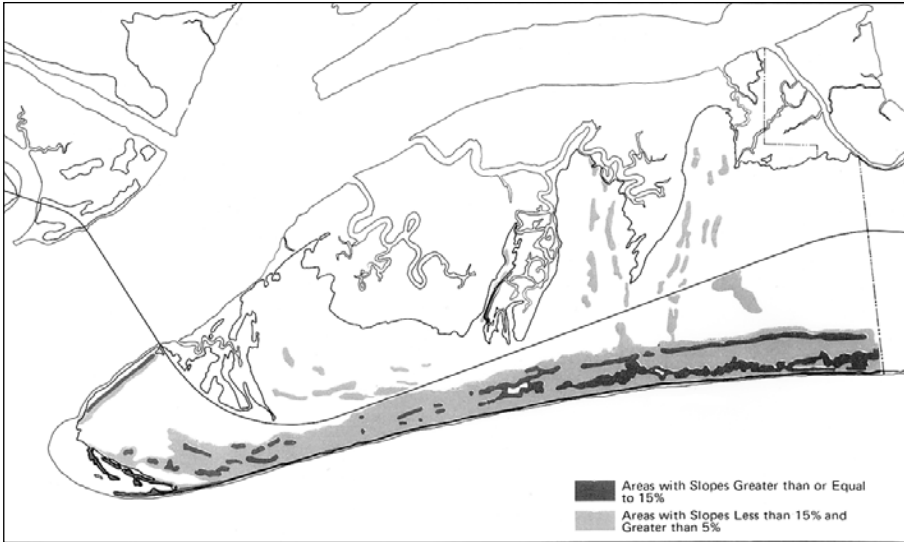
Figures 7.3a–c Ian McHarg’s popularization of the overlay planning method established the basis for rational and scientifically defensible landscape planning. Inventory data such as slope ( A, above ) and tidal inundation ( B, opposite, top ) are assigned values for development and conservation and combined with other data to produce land use suitability maps ( C ). After McHarg, it was generally accepted that the ecology of large territories of land could be mapped and represented in both quality and quantity. © The Architectural Archives of the University of Pennsylvania.
